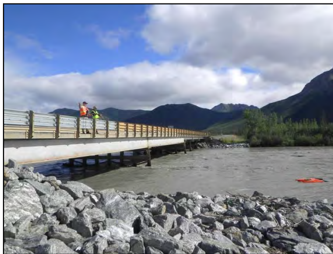
Photo 4 Tethered Deployment of RiverRay ADCP from Bridge on Dietrich River (ST_210.3)
