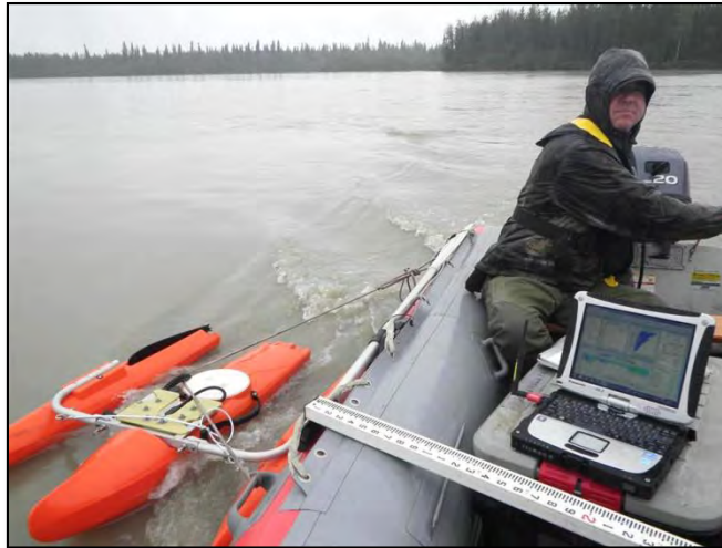
Photo 3 Motorized Boat Deployment of RiverRay ADCP on Tanana River (ST_469.5)
