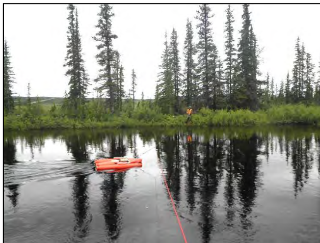
Photo 5 Two Man Tethered Deployment of RiverRAY on Kanuti River (ST_307.9)
