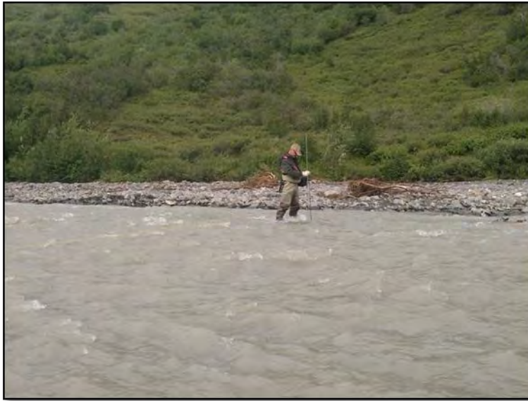
Photo 2 Standard Methods Discharge Measurements using Marsh-McBirney FLO-MATE and Wading Rod on Dietric River (ST_180.4)
